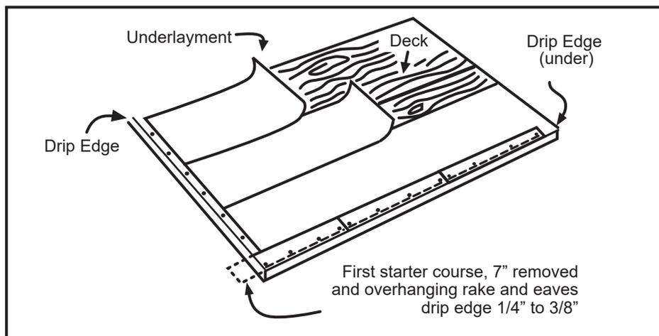
The second starter course is started with a piece of Paramount® Starter matching the color of Cascade™ for the rest of the roof (reference image on page 2). Cut 5" off the length of the first Paramount® Starter shingle and apply it at the lower left corner of the deck, aligned at the eaves and rake with the first starter (overhanging drip edge 1/4" to 3/8").
