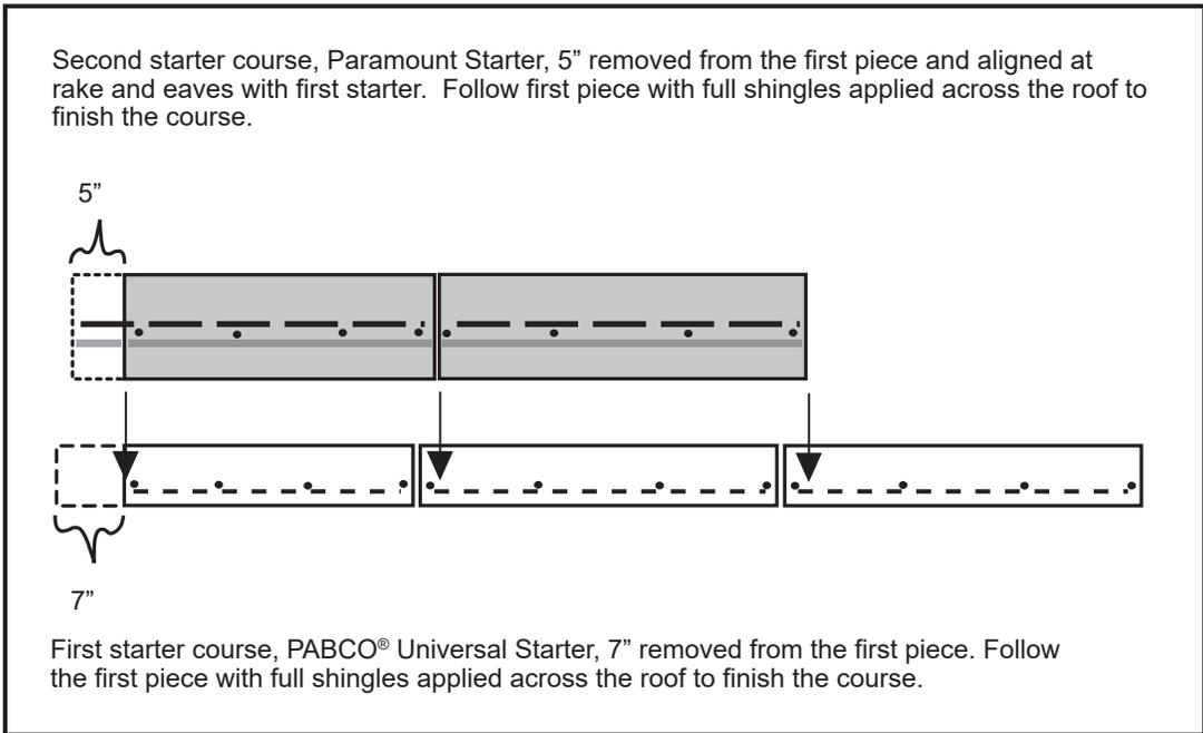
The first Cascade™ course is started with a full length shingle. Place the shingle at the lower corner of the deck, over the Paramount® Starter. Align the end of the shingle and the bottom of the shingle teeth with the edges of the Paramount Starter under it.
