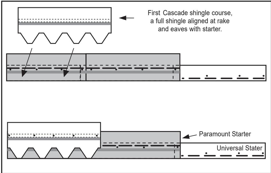
The second Cascade™ course is started with a Cascade shingle with 5" cut off its left end (reference image on page 3). Apply this 35" long piece over the headlap of the shingle below, flush with the left edge of that shingle. The teeth are 4-1/2" high. Expose 4-1/2" of the shingle below by placing the bottom of the teeth for this shingle even with the top of the area between the teeth of the shingle below.
