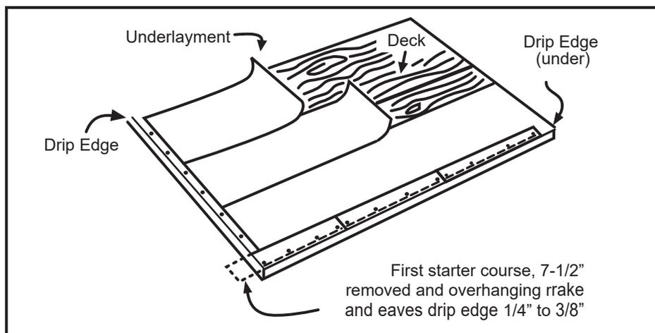
The second starter course is started with a piece of Paramount® Starter matching the color of Paramount for the rest of the roof (reference image on page 2). Remove 5-3/4" from the end. Apply the piece at the lower left corner of the deck, aligned at the eaves and rake with the first starter (overhanging drip edge 1/4" to 3/8").
