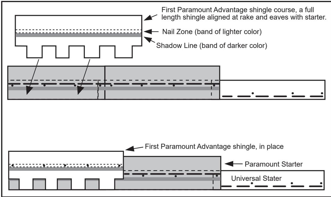
The second Paramount® course is started with a Paramount® shingle with 5-3/4" cut off its left end (reference image on page 3). Apply this 34-1/4" long piece over the headlap of the shingle below, flush with the left edge of that shingle. The teeth are 4-1/2" high. Expose 4-1/2" of the shingle below by placing the bottom of the teeth for this shingle even with the top of the area between the teeth of the shingle below.
