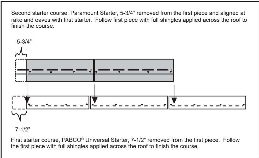
The first Paramount® course is started with a full length shingle. Place the shingle at the lower corner of the deck, over the Paramount® Starter. Align the end of the shingle and the bottom of the shingle teeth with the edges of the Paramount® Starter under it.
